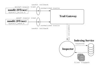
Figure 2. iLeak Prototype Implementation.
