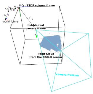
Fig. 1. The voxelized Moving Volume KinectFusion space representation, with the volume transformation frames over time in the initial/world frame.
