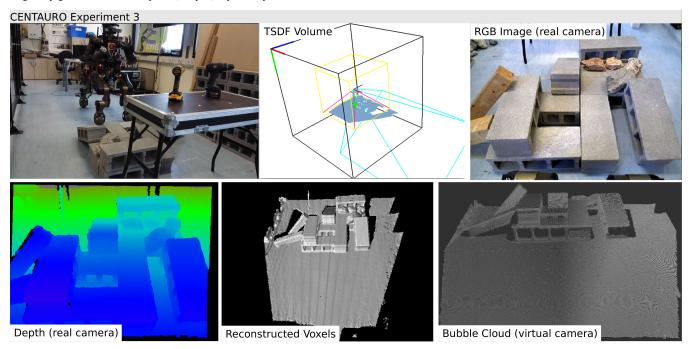
Fig. 9. The experimental results on the CENTAURO robot, including the TSDF volume, the depth/RGB images from the real camera view-point, the reconstructed information from the TSDF voxels, and a dense  $(400px^2)$  raycasted point cloud from the virtual down face of the bubble camera. It is notable that even though the robot stands in front of the rock the raycasted cloud is under its feet.
