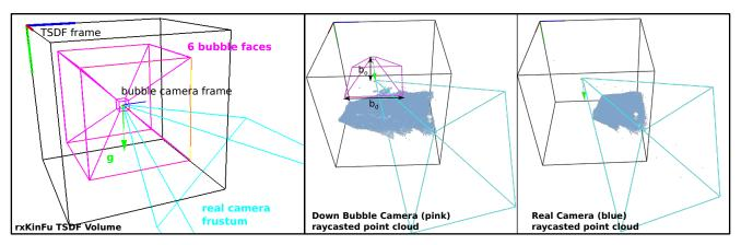
Fig. 3. Left: the proposed rxKinFu TSDF volume, with the 6 virtual bubble camera frustums and the gravity/down vector. Middle: the raycasted point cloud from the down virtual bubble camera after traversing 2m of the trail, using the "Fix Down and then Forward in the Volume (fdv)" strategy and using the gravity as the down vector from an IMU sensor. Right: the raycasted point cloud from the original Moving Volume KinectFusion method.
