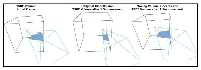
Fig. 2. The original Moving Volume KinectFusion, with the raycasted point cloud from the real camera frustum, compared to the original fixed volume KinectFusion algorithm. The data come from a rocky trail that was crossed with a MS Kinect range sensor, with the instance after 1.5m walking.
