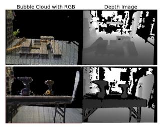
Fig. 4. Left: the raycasted RGB point cloud, from the bubble virtual camera. Right: the depth image of the scene from the real camera.
