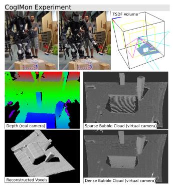
Fig. 7. The experimental results on the COMAN+ humanoid robot, including the TSDF volume, the depth image from the real camera view-point, the reconstructed information from the TSDF voxels, and two raycasted point clouds from the virtual down face of the bubble camera, with different resolutions  $(100px^2 \text{ sparse} \text{ and } 400px^2 \text{ dense})$ .
