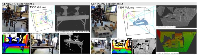
Fig. 8. The experimental results on the CENTAURO robot, including the TSDF volume, the depth/RGB images from the real camera view-point, and the reconstructed information from the TSDF voxels. Left: a dense  $(400px^2)$  raycasted point cloud from the virtual front face of the bubble camera. Right: a heightmap generated from the sparse  $(200px^2)$  raycasted point cloud from the virtual down face of the bubble camera.
