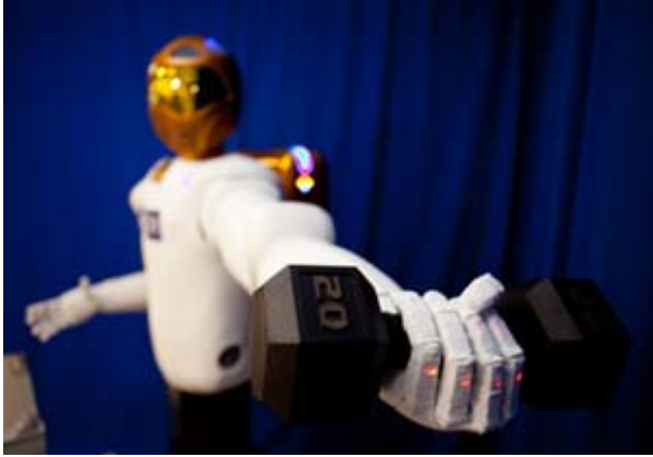
Fig. 3: Robonaut 2 lifting 20 lbs at full extension
