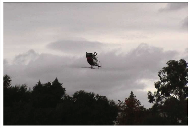
Fig. 7. Autonomous inverted helicopter flight (Ng et al., 2004b). (Reproduced with permission from Andrew Ng.)
