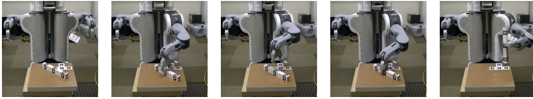
Fig. 4. A recovery behavior when the robot misses the original grasp.
