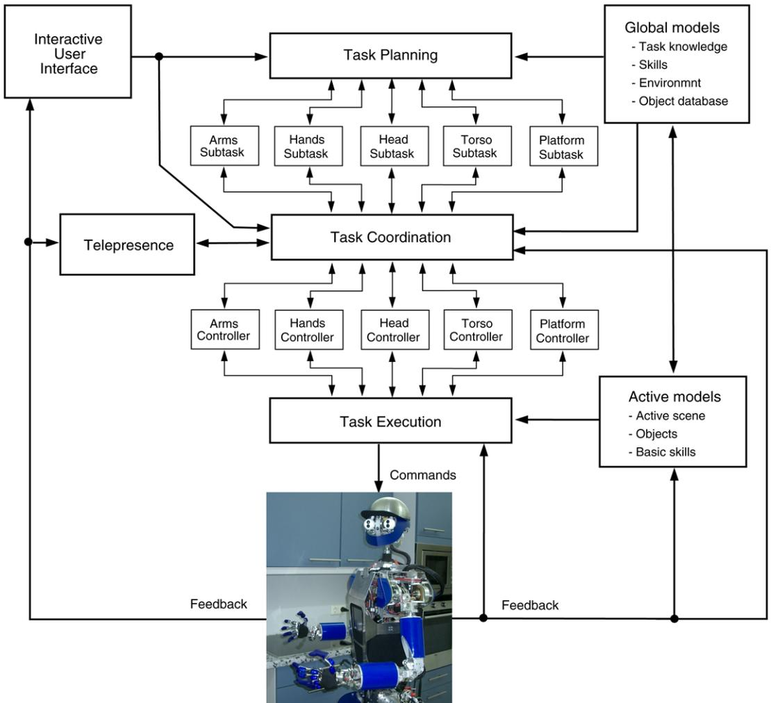
Fig. 2. Hierarchical control architecture for coordinated task execution in humanoid robots: planning, coordination and execution level.
