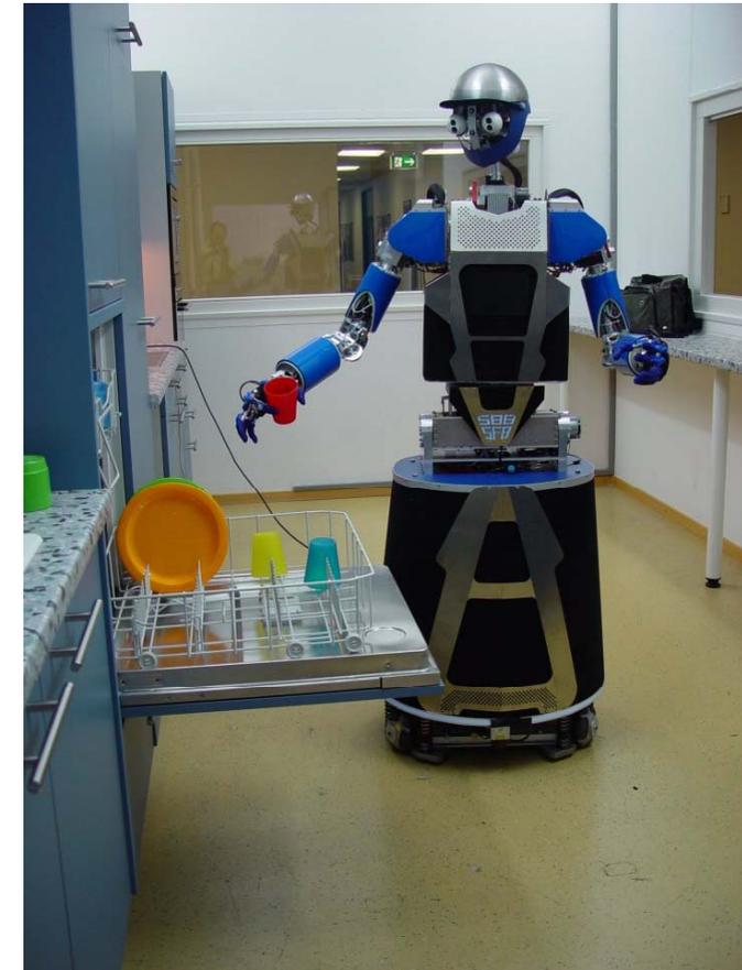
**Fully integrated autonomous humanoid system**
