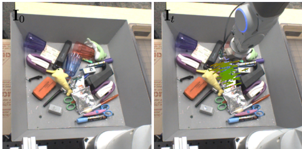
Figure 2. Example input image pair provided to the network, overlaid with lines to indicate sampled target grasp positions. Colors indicate their probabilities of success: green is 1.0 and red is 0.0. The grasp positions are projected onto the image using a known calibration only for visualization. The network does not receive the projections of these poses onto the image, only offsets from the current gripper position in the frame of the robot.
