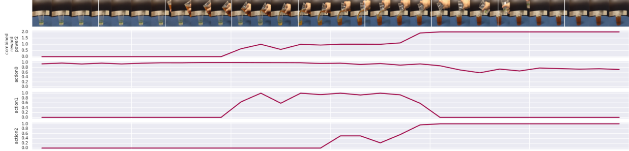
Fig. 9: Combining intermediate rewards into a single reward function. From top to bottom, we show the combined reward function (with range [0,2] ) followed by the reward function of each individual steps (with range [0,1] ). The first step reward corresponds to the initial resting state of the demonstration and is ignored in the reward function. The second step corresponds to the pouring action and the third step corresponds to the glass full of liquid.
