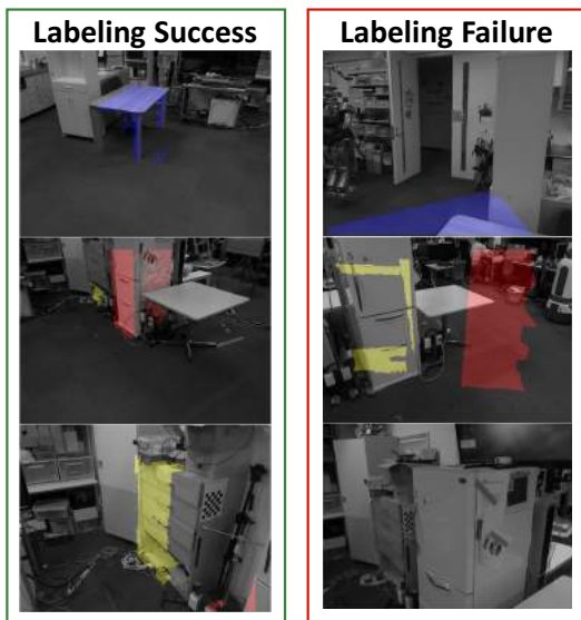
Fig. 4: Dataset generated with our method which is described in Section III. Left side of this figure shows the successfully labeled images, and right side shows the wrongly labeled images.
