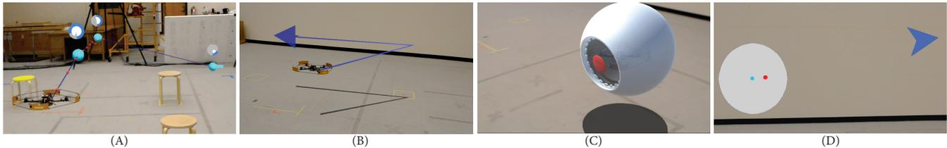
**Figure 1:** In this work, we explore how augmented reality might mediate collocated human-robot interactions by visually conveying robot motion intent. We developed four reference prototypes for cuing aerial robot flight motion: (A) NavPoints, (B) Arrows, (C) Gaze, (D) Utilities.
