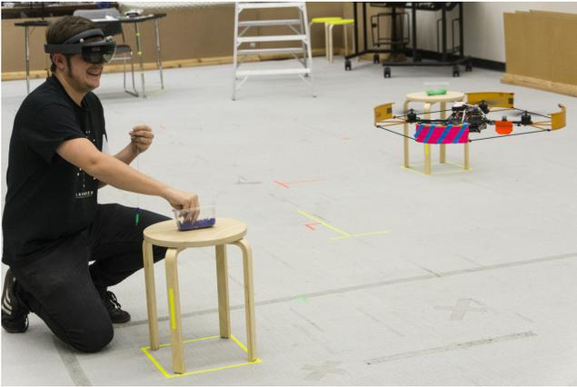
**Figure 3:** Participant making a bead string at one of the six assembly stations mid-task. The AscTec Hummingbird robot flies nearby (colored corner marks robot “front” for baseline participants).
