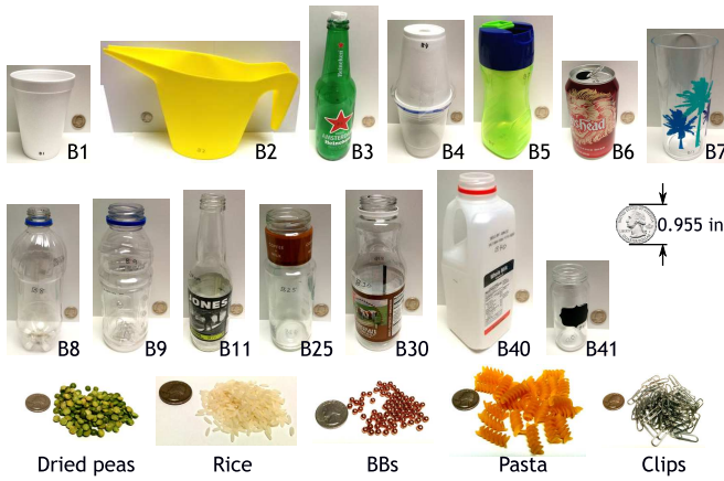
Fig. 8. Source containers and poured materials. Each photo contains a coin of diameter 0.955 inches as a scale. BBs are copper-coated bullets for toy guns. The container B3 and B4 are specially designed for the experiments; these holes are designed to be small in order to produce jamming.
