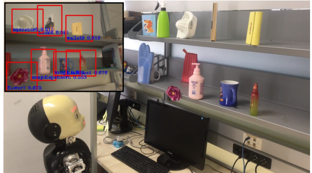
Fig. 1: The iCub robot observes some of the objects learned using the proposed pipeline and detects them on a shelf. A video showing the system running has been made available as Supplementary Material.
