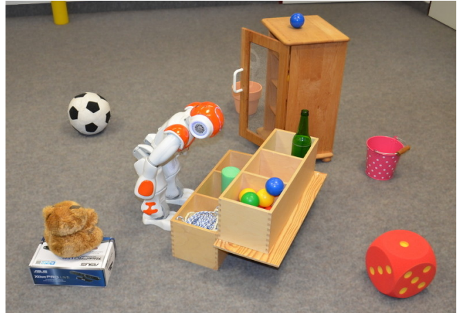
Fig. 1. Nao inspecting an environment. The robot bends over to peek into a box for completing the task of completely covering the environment with its camera, e.g., for finding objects.
