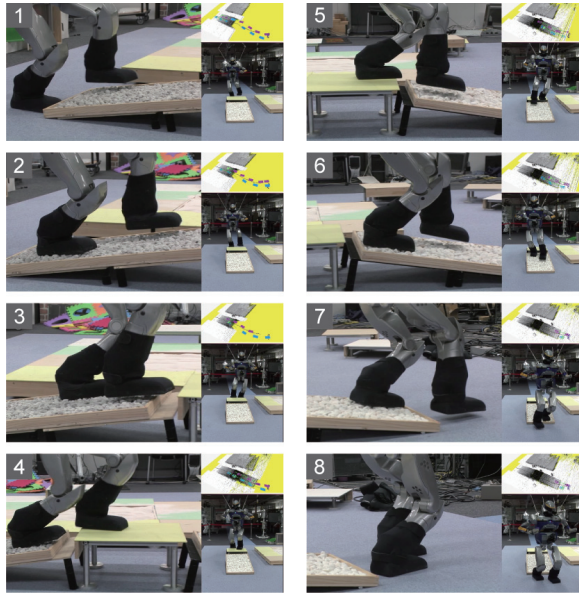
Fig. 16. Photographs of an experiment on autonomous navigation over unknown terrain (GUI) (see also Extension 1).
