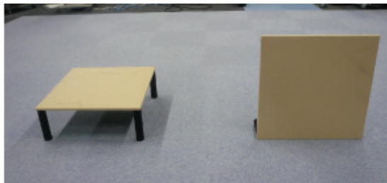
Fig. 5. An example of a terrain with regions of different heights and a wall. (The viewpoint is approximately the same as the position of the laser range sensor from which the data in the following three figures was collected.)
