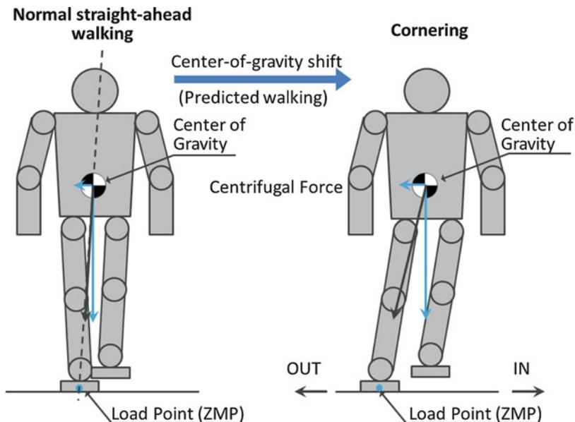
Fig. 12 Center-of-gravity shift
