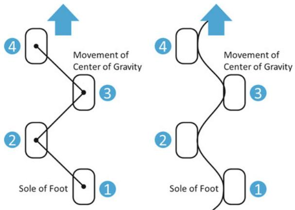
**Fig. 4** Zero moment point
