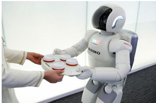
For example, in handing over a tray, the eye camera installed in the robot's head and force sensors in the wrists are used. The camera and the sensors detect the movement of the tray so that the robot can match its actions to the other party and hand over the tray without fail (Fig. 17).
