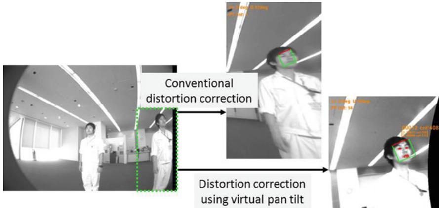
**Fig. 24** Correction of image distortion
