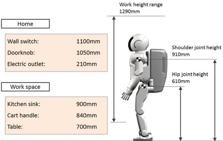
**Fig. 11** Investigation of robot dimension
