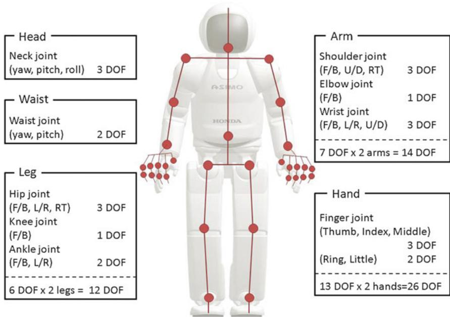
Fig. 25 Joint configuration and DOF (degree of freedom)
