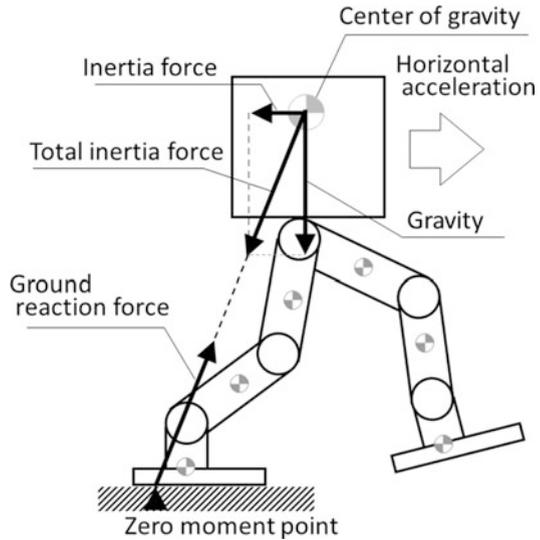
This is accomplished by actively changing the robot's stride length or center of gravity.
