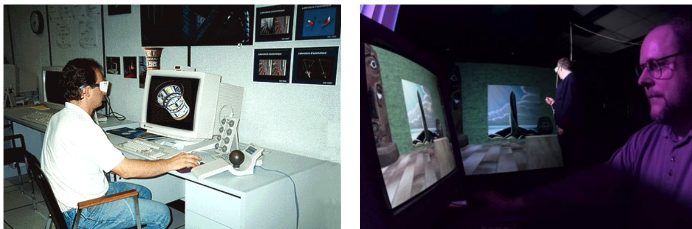
Figure 5. Presenting a 3D scene on a display: a) 3D model of an object is view with stereo glasses and b) a model or a complete environment is experienced in a virtual reality room.
