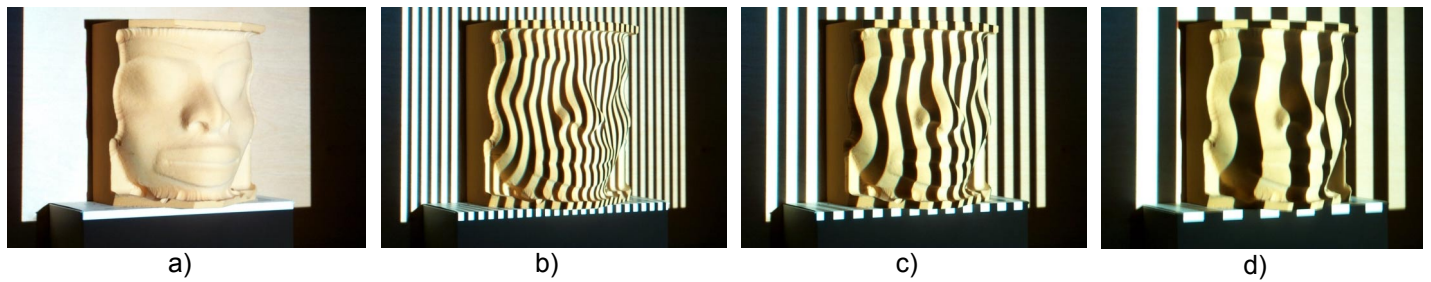
Figure 17. Coded light approach example (the camera is beside the LCD-based projector): a) fully illuminated scene taken prior to projection of the stripe patterns, b), c) and d) grey scale images of the first 3 (usually out of 9) stripe patterns projected with a LCD projector.
