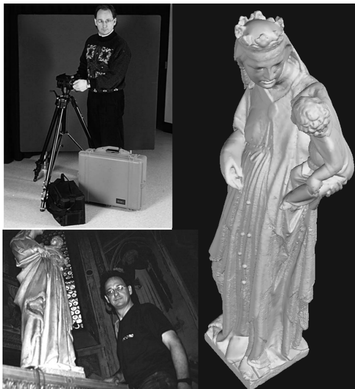
Figure 22. Madonna con il Bambino, G. Pisano (circa 1305): a) portable biris system used to scan the sculpture, b) site in the Cappella degli Scrovegni in Padova, and, c) completed 3D model of the statue shown from a virtual point of view not available to tourists visiting the Chapel. Height is about 1.29 m.
