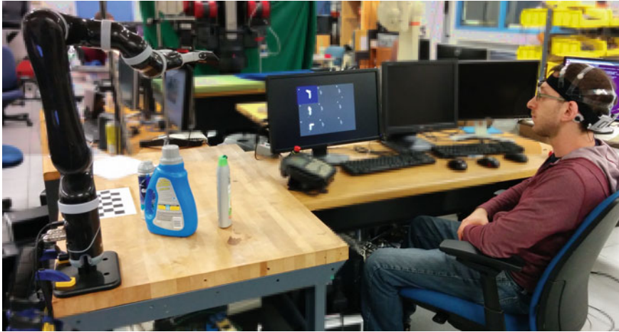
Fig. 1 The subject guiding the system through the active refinement phase. On the left side is the robotic manipulator and three containers in the grasping scene. On the right is a subject using the system through the B-Alert EEG cap, which is relatively unobtrusive and can be worn for long periods of time. The options for the active refinement stage are presented on the monitor in front of the subject in a grid to allow the subject to pick the one they intend to select during the serial presentation. In this example, at least one of the grasps found in the database for the object was reachable, and is highlighted in blue in the upper left corner of the grid. The user may choose to execute the highlighted grasp, or to re-seed the planner with one of the other nine grasps and then re-enter the active refinement phase with a new highlighted grasp
