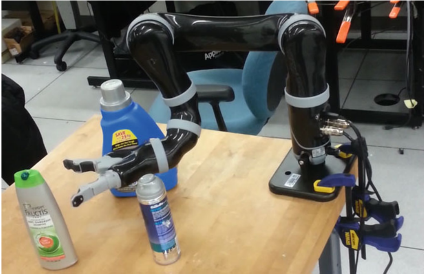
Fig. 5 A typical grasp of the shampoo bottle from the side in the cluttered scene. Note that the hand is just able to fit between the other objects to grasp the desired target. Note that the ability to plan this grasp in such a restricted environment is an indication that this system is very successful at handling the cluttered scene
