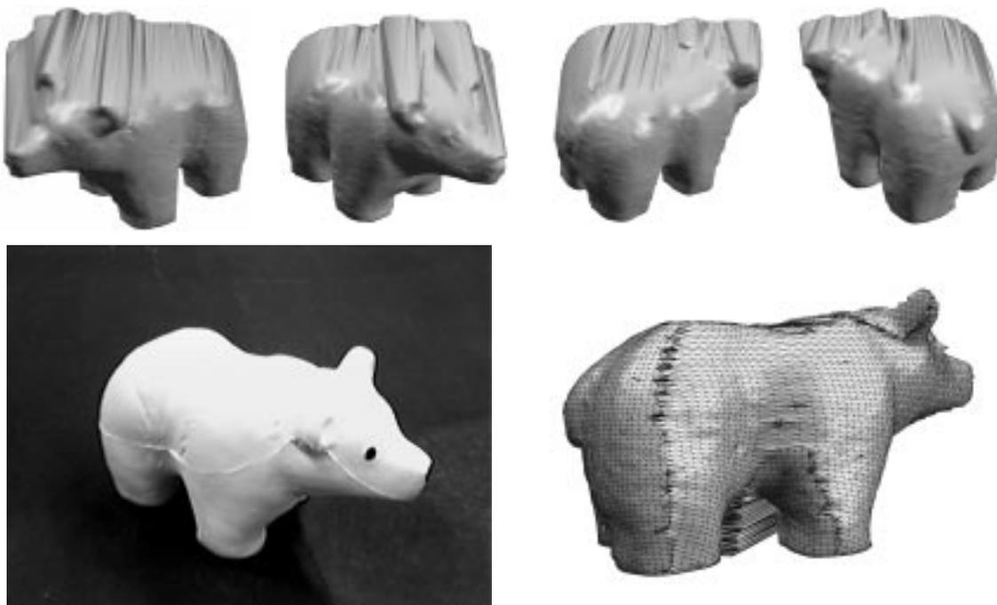
**Figure 3-22. Models of the toy bear in four views. The solid models from four distinct range images are shown, as is the wireframe of the composite model next to a photograph of the actual object.**
