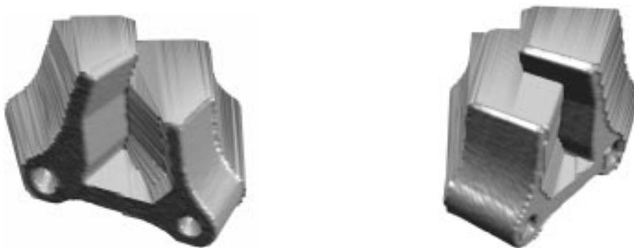
**Figure 4-18. Initial models from strut acquisition. The solid models constructed by sweeping the mesh surface of the first two range images are shown.**
