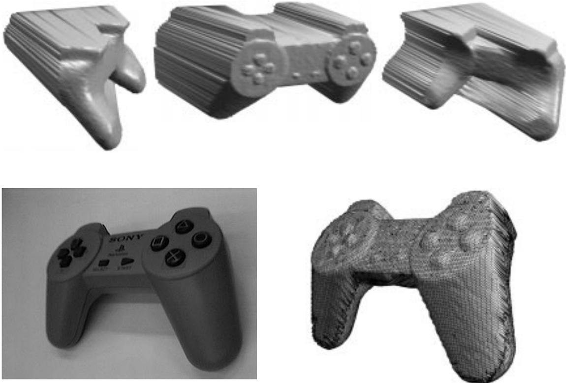
**Figure 3-23. Model of the video game controller in three views. Solid models from each of three views are shown at top, bottom left is photograph of actual part, bottom right is wireframe of acquired model.**
