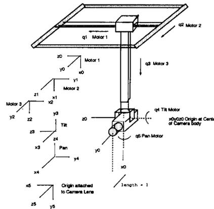
Figure 1: 5-DOF Hybrid Robot
