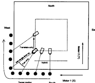
Figure 6: Kinematic Constraints Handling
