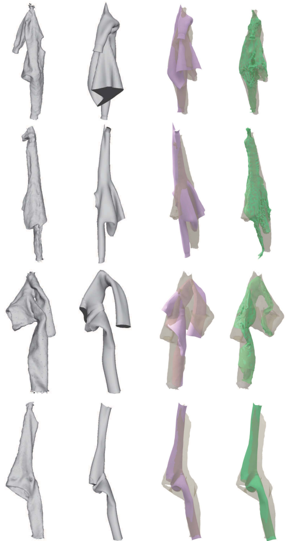
Fig. 14. Registration examples. First row: sweater grasped at elbow. Second row: long-sleeve shirt grasped at sleeve end. Third row: pair of pants grasped near knee. Fourth row: pair of pants grasped near ankle. Each row depicts from left to right: reconstructed mesh, predicted mesh from the database, rigid registration only, and rigid plus nonrigid registration.
