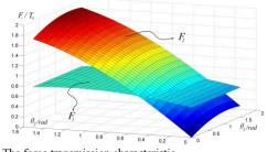
Fig. 5.The force transmission characteristic Notes: in this figure, the contact point is fixed,  $k_1=k_2=(L_1+L_0)/2$ ; and all the other design parameters are the same as the specified design which will be discussed later; the range of both angles is from 0 to  $\pi/2$ .
