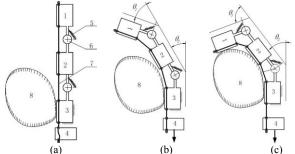
Fig. 1.The principles of a tendon-pin under-actuated finger, illustrating (a) the initial stage, (b) the pre-shaping stage, and (c) the closing stage. Notes: 1 – the distal segment; 2 – the middle segment; 3 – the fixed segment; 4 – the lifting mechanism; 5 – the return spring; 6 – the joint pin; 7 – the tendon; 8 – the grasped object
