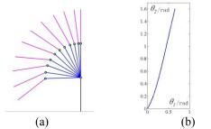
Fig. 3. The relationship between  $\theta_1$  and  $\theta_2$ , demonstrating the ability to predict the pre-shaping position as well as a strong resemblance to human movement.(a) simulates the pre-shaping while (b) shows how the two angles are coupled. Both analyses are done with the same parameter configuration as the specified design which will be discussed later, and the pre-loading torque is set to zero for convenience.
