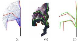
Fig. 11. Results of the pre-shaping test with an individual finger: (a)shows the animation computed from sensory feedback while (b)shows the ground truths; (c) compares the first, middle, and last positions of (a) and (b). These demonstrate a high degree of accuracy of the position feedback system and a natural preshaping process strongly resembling the prediction above.
