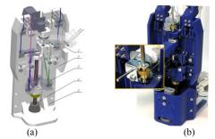
Fig. 7.Actuation system design featuring a single lead-screw mechanism for the tendons and a non-backdrivable motor for the thumb rotation. Notes:1 – the thumb;2 – palm;3 – the lifting mechanism;4 – the lead screw transmission;5 – the wrist frame
