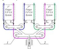
Fig. 6. The movable block mechanism, which allows all three fingers to be controlled by a single motor but still conform to an arbitrary object shape. Notes: 1 – the movable pulley; 2 – the rigid frame;  $T_{kj}$  e.g.  $T_{lb}$  – the tendon force produced by the blue tendon in the figure;  $T_{\Sigma}$  – the force applied on the frame (produced by the lead-screw mechanism).
