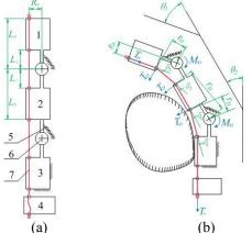
Fig. 2. The mechanical analysis of the pre-shaping stage Notes: 1 – the distal segment; 2 – the middle segment; 3 – the fixed segment; 4 – the lifting mechanism; 5 – the return spring; 6 – the joint pin;
