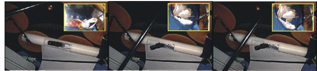
Fig. 5. Another task, that required motions over greater distances, was performed within the training box. Again the assistant was able to keep the activity within the field of view of the camera. This sequence more clearly shows the motions of the camera.
