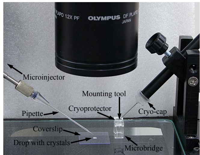
Fig. 4. A closeup of the workspace showing the pipette attached to the micromanipulator and the microinjector on the left side and the mounting tool attached to the receptor fixture on the right side of the microscope objective.
