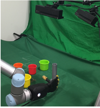
Fig.2: Pick-Pour-Place Robot Setup at Test Time. Given an RGB image from the top-down (black) or 45° camera (also black), the UR5-Seed robot is tasked to approach and pick-up the grey cylindrical bottle, pour the iron pebble already inside the bottle into a specific container on the table and finally place the bottle back on the table.
