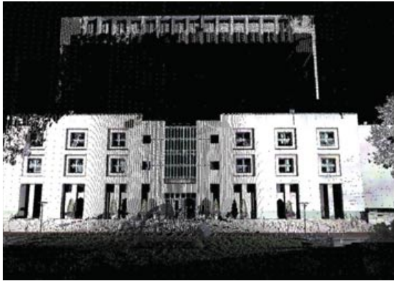
Figure 16. Left: The facade of Uris Hall, scanned from the views generated by the Phase I planner. Phase I generated views only at the corners of the building, causing much of the tower to be occluded by the base. Right: The facade of the same building after acquiring the first NBV.
