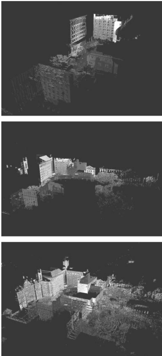
Figure 15. The initial campus model being constructed sequentially from the 2-D plan. From top to bottom: The first scan, registered scans 1–4, and the complete initial model with all nine scans. The scans are texture mapped with images taken from the scanner’s built-in camera. (These images are best viewed in color.)
