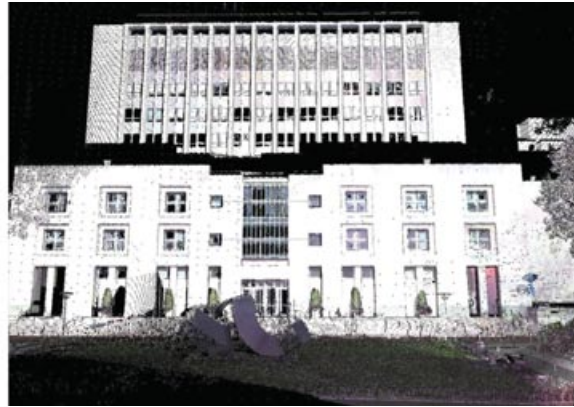
Figure 16. Left: The facade of Uris Hall, scanned from the views generated by the Phase I planner. Phase I generated views only at the corners of the building, causing much of the tower to be occluded by the base. Right: The facade of the same building after acquiring the first NBV.
