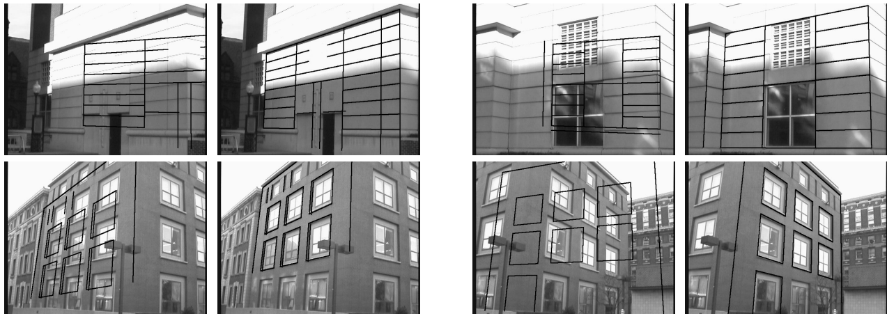
Figure 7: Initial and final alignments in the pose estimation tests with a pair of images taken from the same location.
