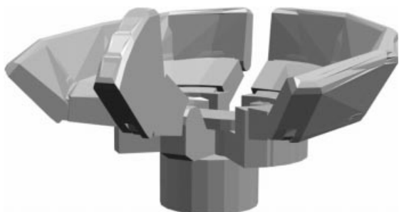
Figure 14. Computed swept volume of a Barrett hand, closing.
