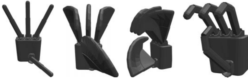
Figure 16. Left: initial configuration of the DLR hand. Centre: front and side views of the swept motion of the links. Right: final configuration of the hand.
