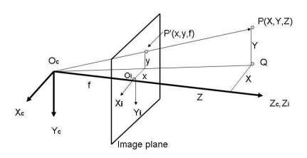
Figure 1: Perspective imaging geometry showing relationship between 3D points and image plane points.
