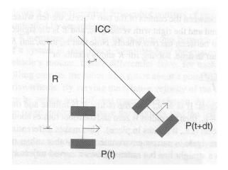
Figure 2: Forward kinematics for differential robot
