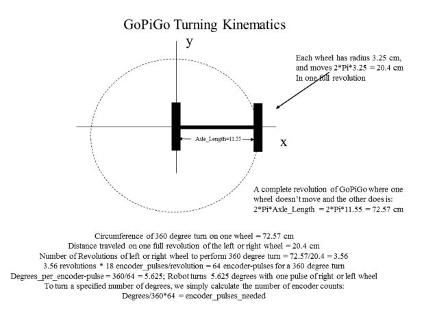
Figure 3: GoPiGo wheel kinematics
