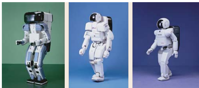
Fig. 56.6 Honda P2 (180 cm tall, 210 kg), P3 (160 cm, 130 kg), and Asimo (120 cm, 43 kg) [56.26]. (Images courtesy of Honda)
