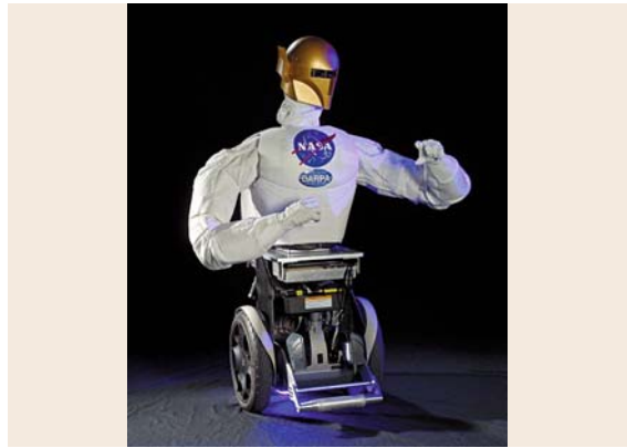
Fig. 56.8 The NASA Robonaut consists of an upper body placed on a wheeled mobile base
