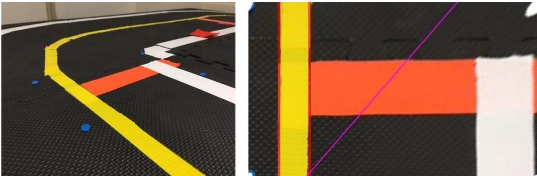
Left: Here is another image taken from an angle. Right: the homography and the mapping of the robot's direction of travel onto the grid. The angle between the magenta line and the red hough line on the yellow centerline can be used to re-orient your robot to move parallel to the centerline. The magenta line is calculated by taking the vertical line in the middle of the original image and transforming it with the homography matrix into a line whose coordinates are now in the roadway grid.
