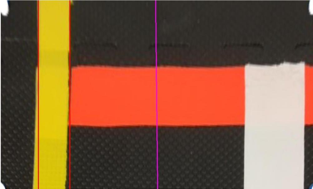
Hough transform line detector (red lines) overlaid on roadway image. The magenta line is the orientation (direction of travel) of the robot relative to the grid when the picture was taken. If we extend this line back from the bottom of the image we can also find out the robot's position on the roadway.
