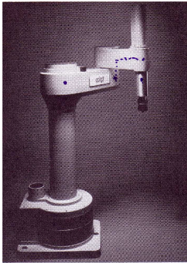
Figure 2: Adept 1 Scara Robot arm. This arm is in a R-R-P-R configuration. \theta_1, \theta_2, \theta_4 are the revolute joint angle variables and q_3 is the prismatic joint variable. The robot is pictured in the Home position in the frame diagram using the values of the joint variables listed in the table below.
