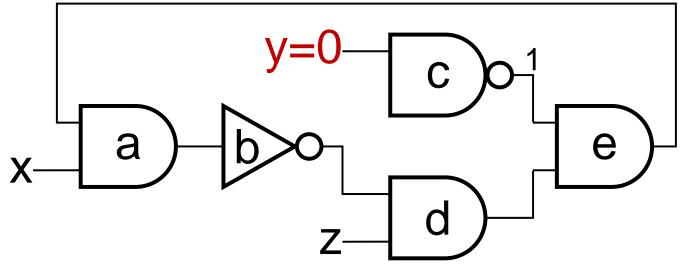
The three inputs to this are x, z, and the output of gate c.
