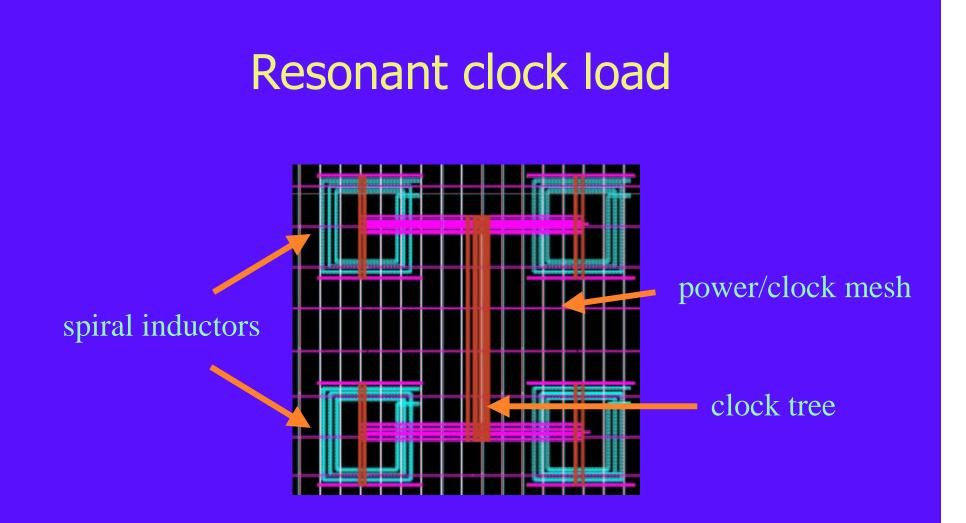
Traditional tree-driven grid augmented with spiral inductors to resonate the clock capacitance at the fundamental of the clock frequency.
