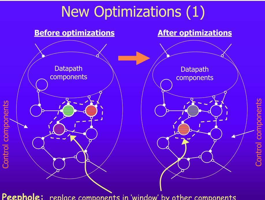
Peephole: replace components in 'window' by other components
