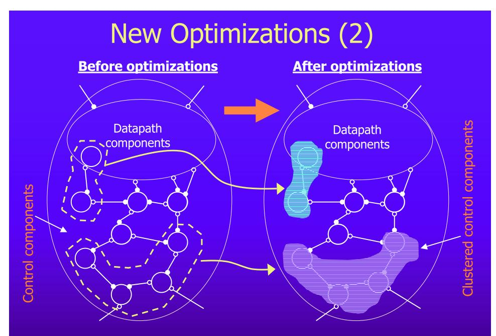
**Resynthesis:** <u>cluster together</u> components (both control and datapath)
