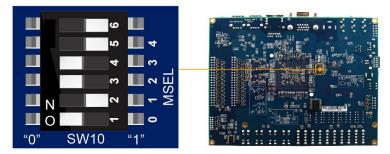
For this lab, we will be configuring the FPGA with a JTAG interface through USB; the Active Serial mode makes the board start up in a factory demonstration mode.
