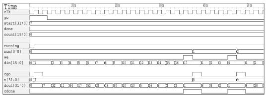
The *go* input switches *running* to true; loads *n* with the value on *start*; resets *num*, the RAM address, to 0; sets *din*, the iteration count, to 1; and pulses *cgo* high for a cycle to start the Collatz iterator module.
