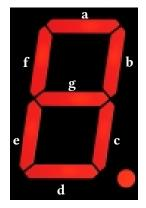
Implement the body of the sevent-segment decoder module in *hex7seg.sv*. We have provided a Verilator testbench to test your implementation. Make sure Verilator is installed and compile and run the simulation:
