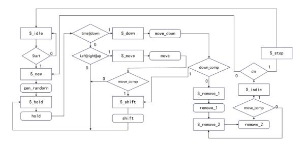
Figure 2: Finite State Machine
