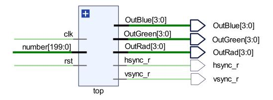
Figure 4: VGA Module
