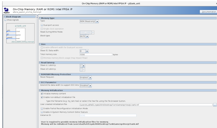
Figure 2.1a: ROM configuration in Platform Designer
