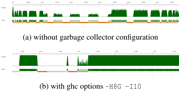
Figure 4: Threadscope visualizing event traces of sequential Varys running on a single HEC, with and without tuning GHC runtime options of garbage collector.
