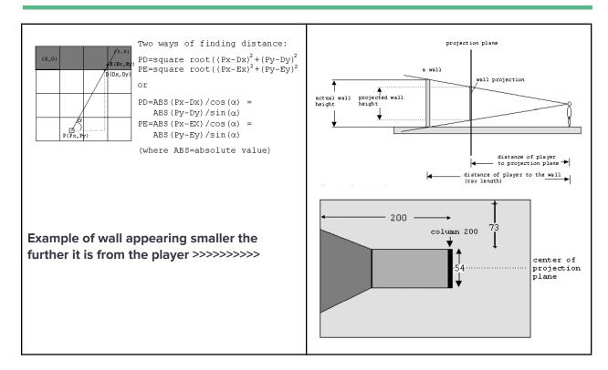
This highlights the algorithm. There are additional manipulations to prevent fish bowl effects, adding textures to the walls, drawing floors and the sky, moving forward, backward, but the rendering algorithm continues to use the above computations.
