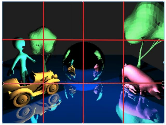
However, there's a pitfall in this case that the first 3 blocks barely need any execution time, as there's almost nothing in that area. As a result, the task to be heavily unbalanced and lead to notably longer execution time.
