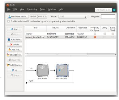
Finally, click on "Start" to program the FPGA. This should quickly report "100% (Successful)" on the programmer.
