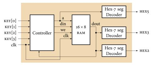
Implement a memory display and modification circuit according to the block diagram above. The circuit should always display the address and contents of one of 16 byte-wide memory locations.
