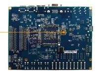
For this lab, we will be configuring the FPGA with a JTAG interface through USB; the Active Serial mode makes the board start up in a factory demonstration mode.
