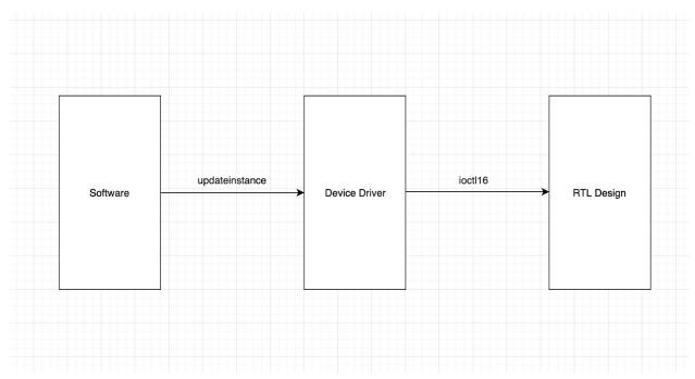
In this part, the software will pass a bunch of parameters required for vga displays to the device driver and the device driver will then give them to the hardware via ioctl16. Below is a table of registers required by each object.
