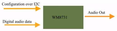
Fig.7 Block diagram of WM8731 CODEC
