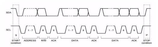
Fig.8 Timing of I2C interface
