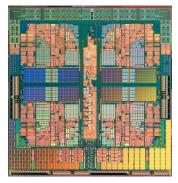
AMD Phenom 9600 Quad-core 2.3 GHz 1.1–1.25 V 95 W 65 nm
