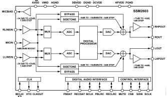
Two 24-bit ADCs; two 24-bit DACs + 7 mW headphone amp Sampling rates: 22.05, 24, 32, 44.1, 48, 88.2, and 96 kHz
