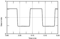
Source: Stereophile magazine: Marantz SM-11S1, small-signal 10kHz squarewave into 8 ohms. A \$4000 audiophile amplifier rated 5 Hz–120 kHz.
