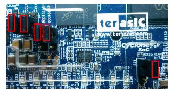
Power on the board. After a few seconds, start the *screen* terminal emulator on the desktop workstation by typing in a shell window
