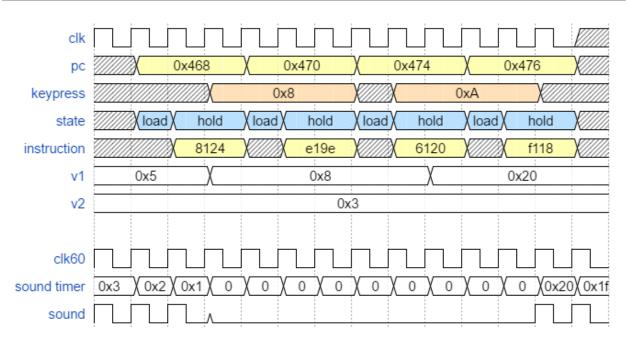
Figure 7: Chip8 example program timing diagram
