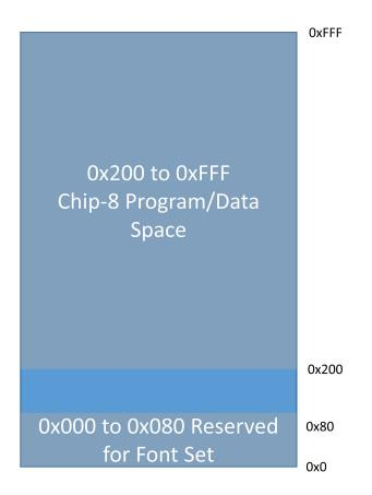
Figure 2: Chip8 4K memory layout
