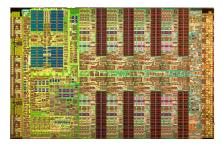
Intel Quad Core Duo Four identical x86 processor cores
