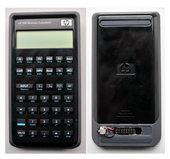
Figure 1: The front and back of the HP 20b calculator. I cut a hole and added the JTAG header so we could develop software on these.
