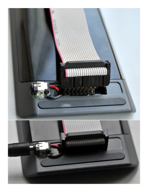
Figure 3: Connecting to the development ports on the back of the HP 20b calculator. Note that the JTAG connector extends beyond the header and we are not using the external power jack.
