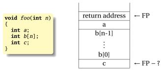
Doesn't work: generated code expects a fixed offset for c. Even worse for multi-dimensional arrays.
